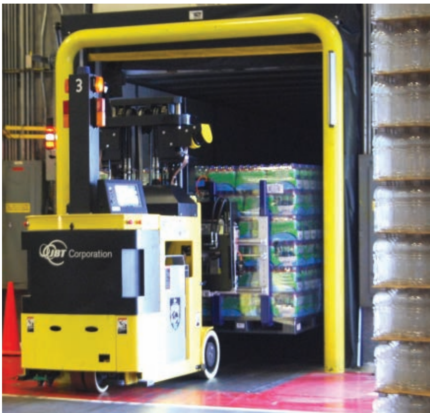
A 5,000-pound capacity, counterbalanced automatic guided vehicle system loads trailers in multiple patterns.
